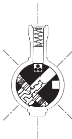
Change key rotating. Construction balls fall into hole in the side of plug.
