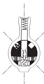
Change key rotated to position for extraction. Construction key now voided from cylinder.
